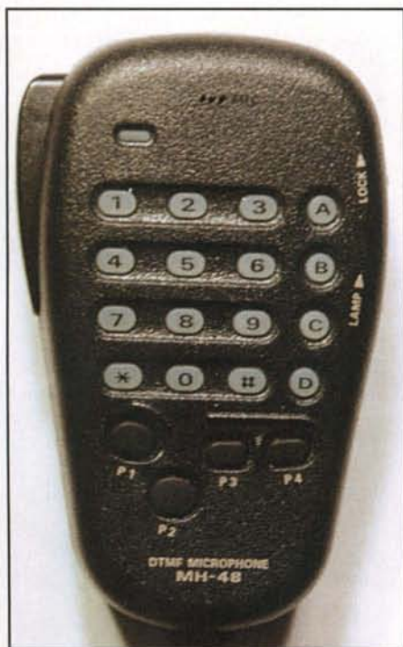
Most mobile transceivers implement the DTMF keypad on the microphone. Shown here is the Yaesu MH-48.
