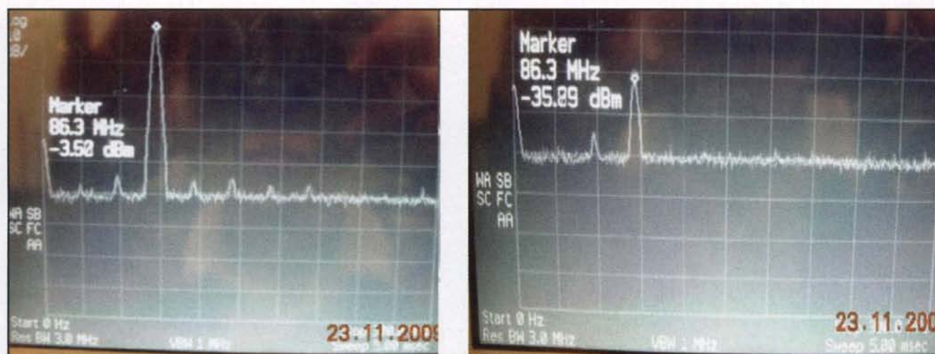
Figure 12. The output of 86-MHz intermediate frequency module with the extremes of input signal.
