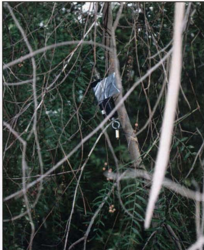
For beginner transmitter hunts, I use 50-milliwatt "Squawk-box" transmitter boards from Bob Simmons WB6EYV < http://www.silcom.com/~pelican2/PicoDopp/MICROHUNT.htm >. They are programmed to transmit a voice message and ID at frequent intervals. I put them in chalkboard-eraser-size plastic boxes with locking devices made from piano wire to prevent theft. Attached to a sturdy branch in a tree or bush, they can't be spotted at a distance.
