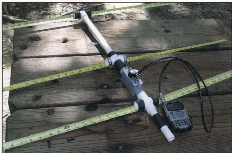
This measuring-tape Yagi with offset attenuator in its boom was assembled from Marvin Johnston's kits.
